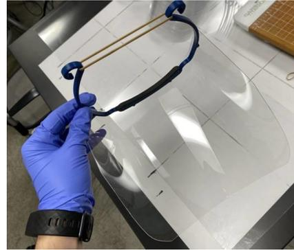
Once the headband pieces are printed, LVO volunteers assemble the face shields by adhering foam strips on the inside of the headbands for the wearer's comfort, attaching the pre-cut and hole-punched clear shields, and adding the adjustable bands to provide a custom-fit for each end user.
